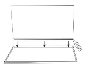
Step 1: Apply glue along the bottom edge of the back wall and set it into the channel inset in from the back of the base.
