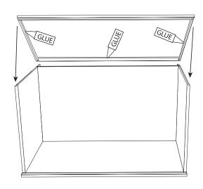
Step 3: Apply glue inside the channels on back and sides of the top and fit onto the top of the box. DO NOT put glue in front channel of top.
