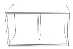
Step 5: The extra piece of solid MDF with no grooves can be used as a divider to make the box into two rooms.
