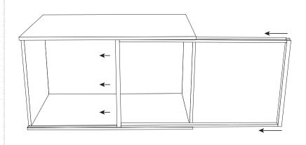
Step 4: Slide the assembled section with pane from the side into the top and base front grooves. DO NOT GLUE. This panel allows access from the front.
